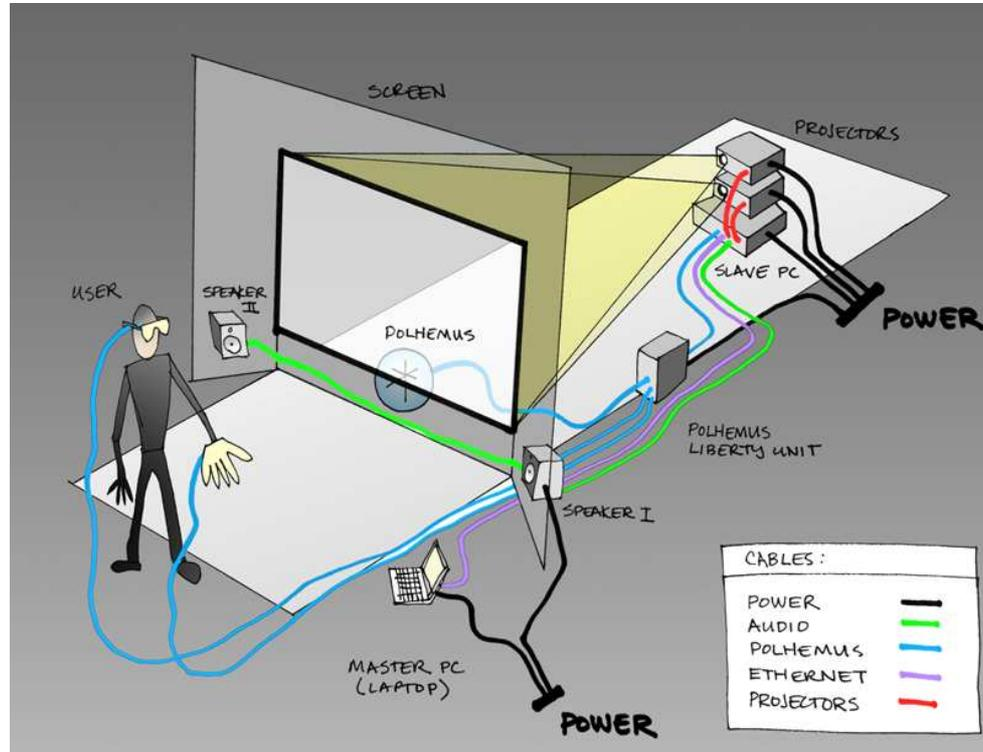
**figure 3.** Installation overview: technical components for "Passages"
